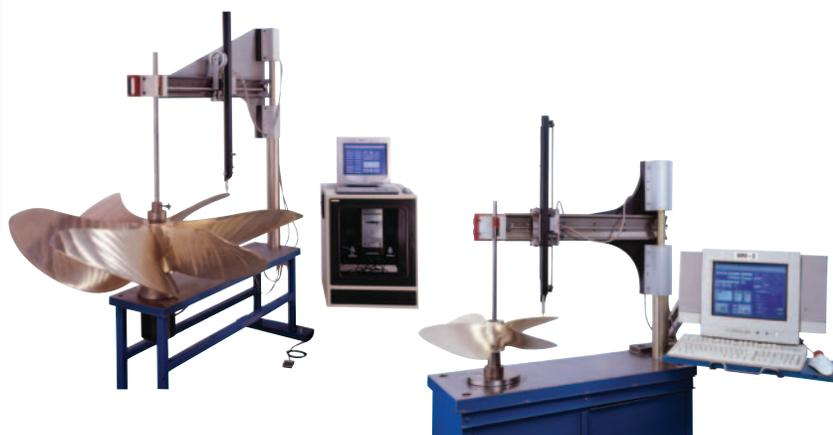
In process and final inspection with gauges, pitchometer, and computerized inspection (MRI), equipment insures production accuracy.
