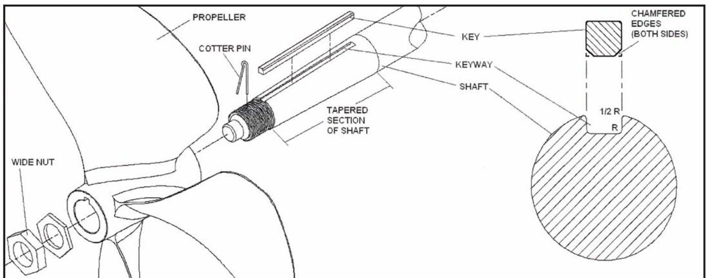
APPROVED S.A.E. STANDARD DIMENSIONS FOR SHAFTS 3/4 TO 3 INCHES IN DIAMETER
