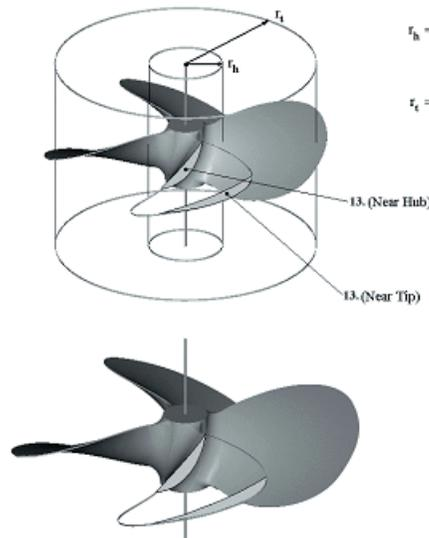
$r_h$  = The radius of a cutting cylinder near the hub. The cylindrical section near the hub is located on the surface of this cylinder.
