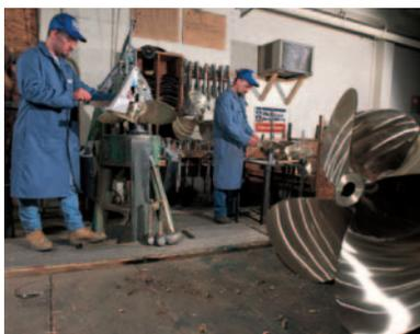
Each hand-crafted or machine finished propeller blade is templated, and each propeller is checked for pitch, spacing and track in process, to insure accuracy of the final product. Balancing equipment is located and used in each step of the finishing process.
