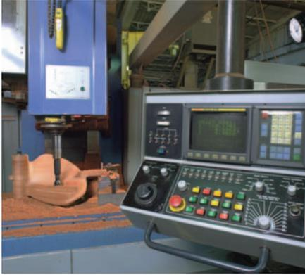
From design to final finish, Michigan Propellers has complete pattern making capacity, in wood, metal and plastic.
